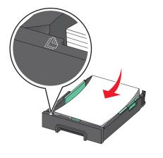
**9** Adjust the paper guides to rest against the left, right, and bottom edges of the paper.
